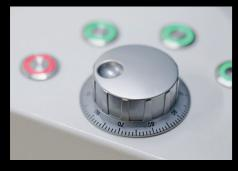
Control is facilitated by a wheel for activating the digitized axes and by four control buttons for function activation and diameter correction in steps of +/-0.001 and 0.0001.
