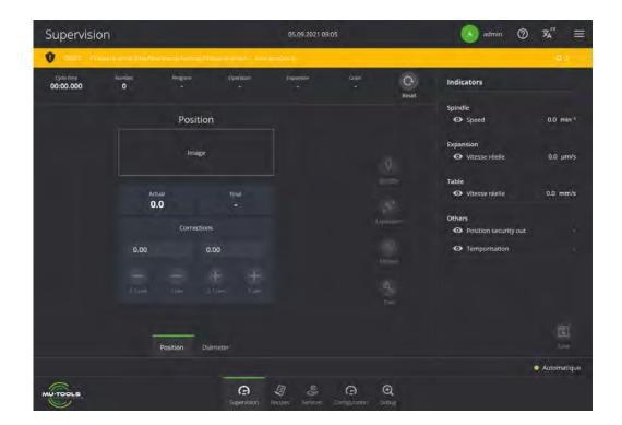
The Beckhof control panel allows several hundred programs to be saved and also allows programs to be exported or imported into an external system.
