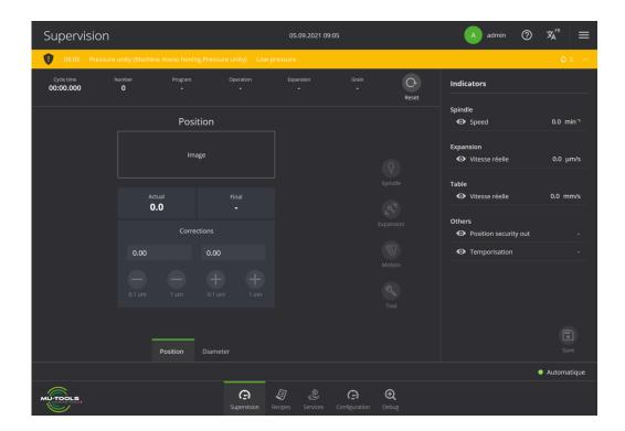
The Beckhof control panel allows several hundred programs to be saved and also allows programs to be exported or imported into an external system.
